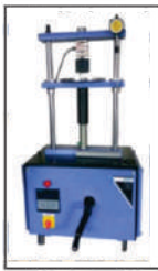
Compression Testing for Mechanical Strength
